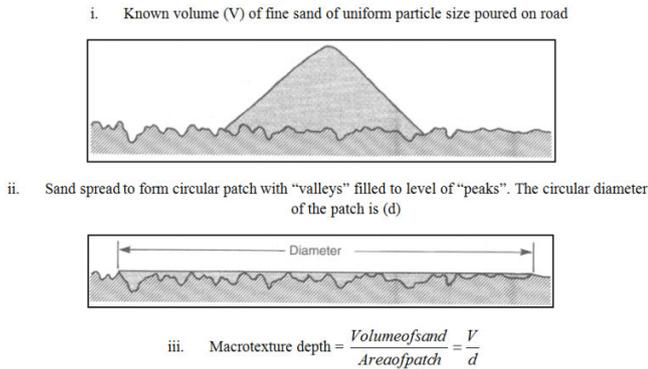
Fig. 5 Illustration of the sand patch method
