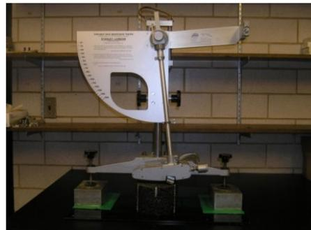
Fig. 4 Friction measurement setup using the BPT
