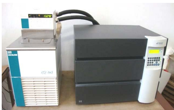
Fig. 3 Apparatus Holometrix 2300 for determination of thermal conductivity
