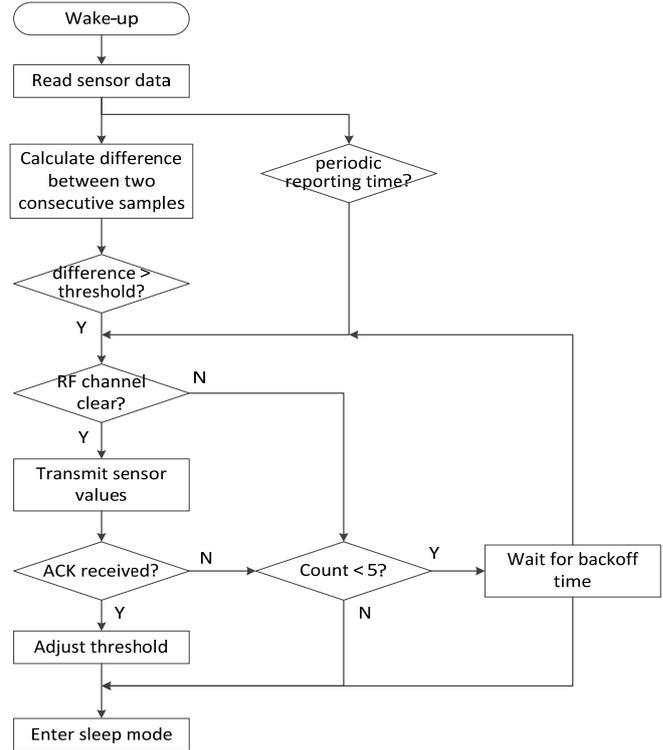
Fig. 5 Operations executed by the sensor node after wake-up
