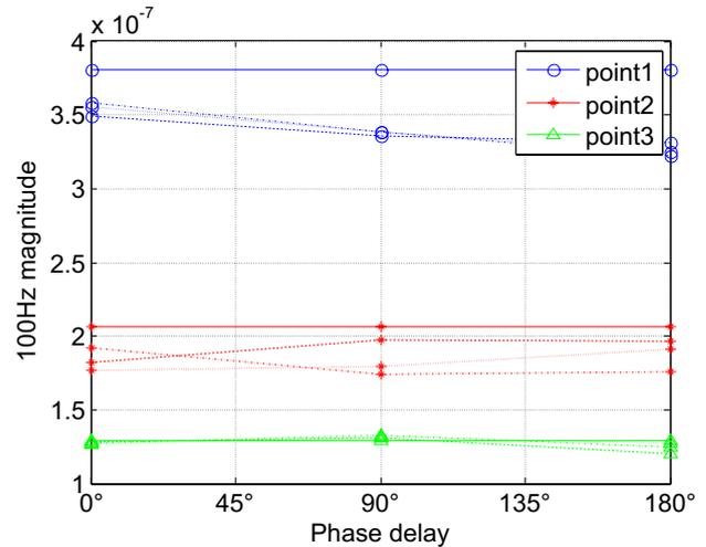
Fig. 3. The 100Hz magnitude [m] of the selected points measured by the scanning laser vibrometer under a purely sinusoidal magnetic induction ( $B=1.2T$  and  $f=50Hz$ ) and a sinusoidal magnetic induction with a third harmonic component with 6%, 8% and 10% amplitude ratios and  $0^\circ$ ,  $90^\circ$  and  $180^\circ$  phase delays with respect to that of the fundamental.
