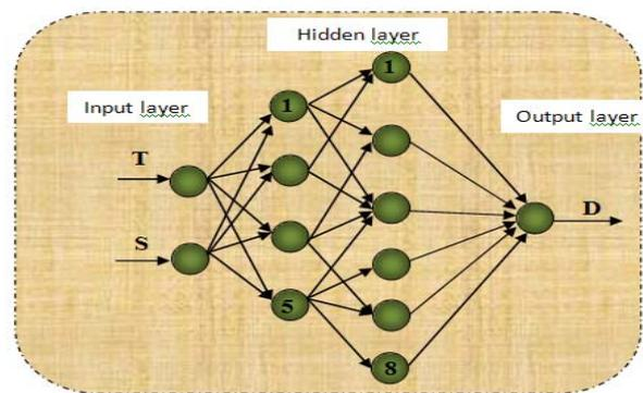
Fig. 4 The proposed neural network architecture
