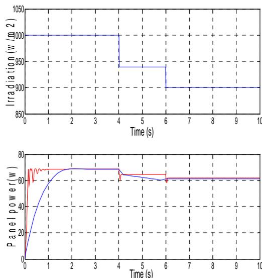
Fig. 9 Output power of PV for different irradiation
