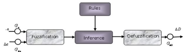
Fig. 5 Basic structure of fuzzy logic control
