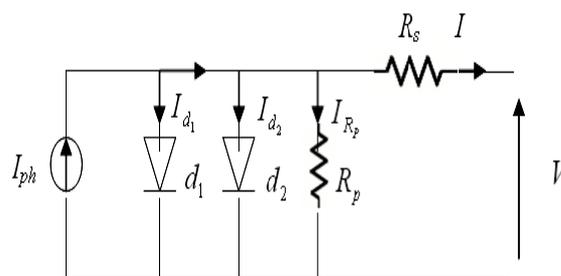
Fig. 1 Equivalent electrical circuit for the PV cell
