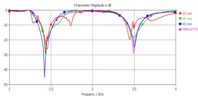
Fig. 7 The  $S_{11}$  of dual band antenna
