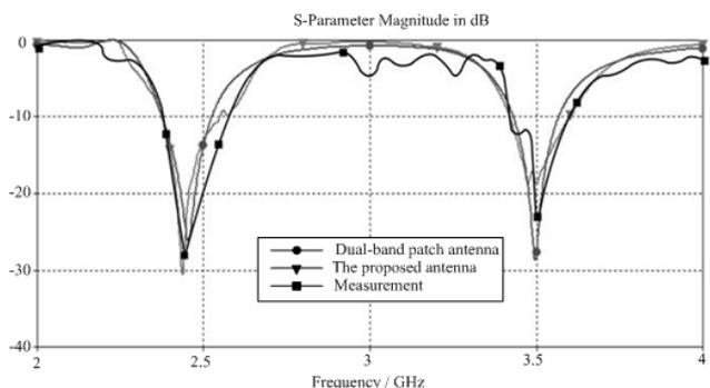
Fig. 9 Comparison of simulation and measurement return loss
