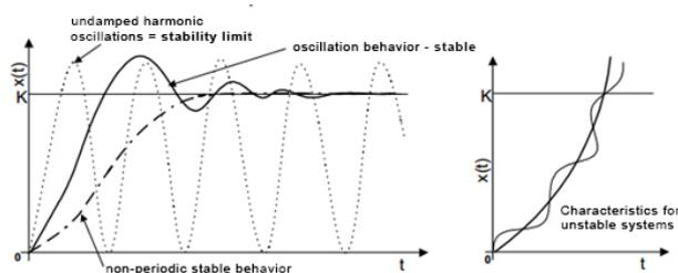
Fig. 2 Example of stable system transfer function
