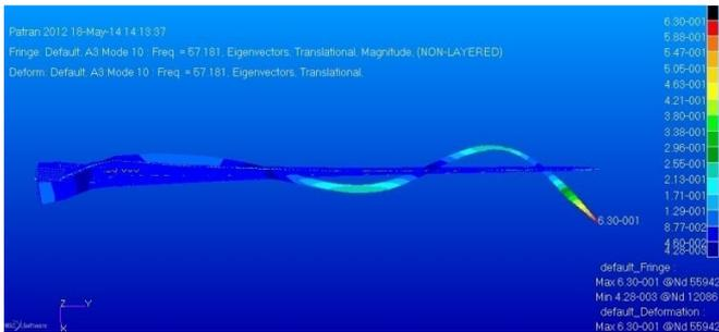
Fig. 21 3<sup>rd</sup> Out-of-plane Bending [57.18 Hz]
