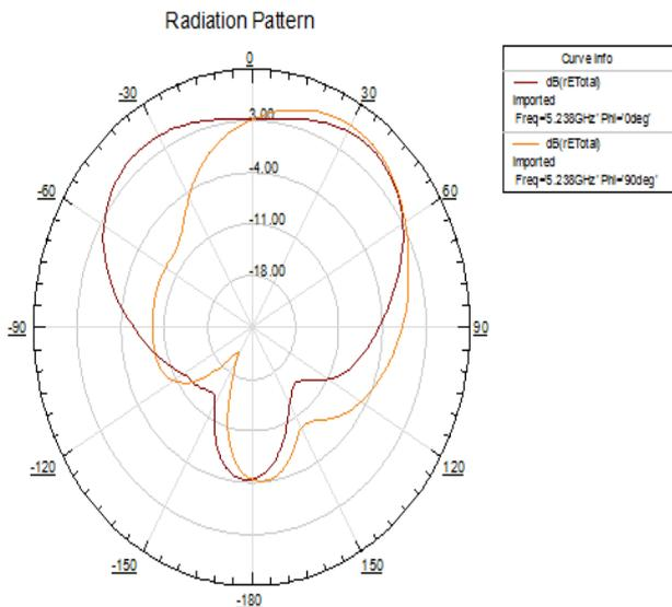
Fig. 3 (e) Simulated radiation pattern at 5.238 GHz
