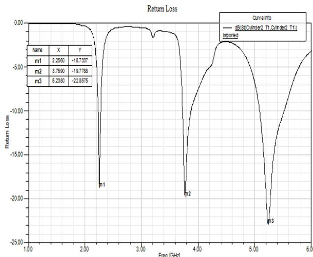
Fig. 3 (a) Simulated return loss for proposed antenna
