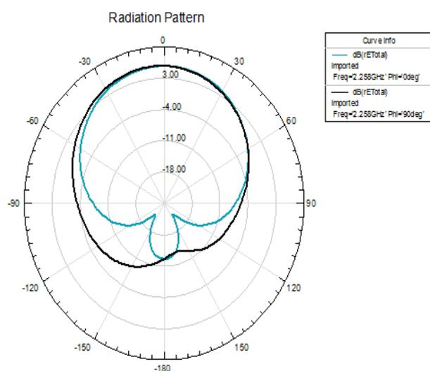
Fig. 3 (c) Simulated radiation pattern at 2.256 GHz
