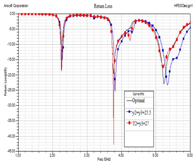
Fig. 7 Simulated return loss for different values of 'y2' & 'y3'
