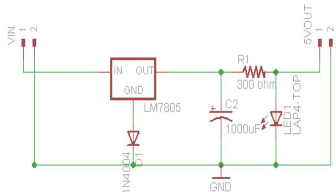
Fig. 7 Schematic of 5 Volt voltage regulator
