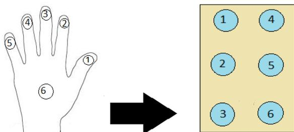
Fig. 1 Comparison between Hand glove and Braille cell
