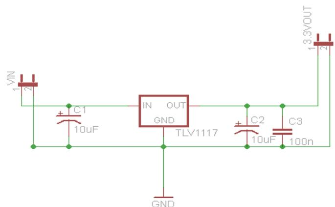
Fig. 8 Schematic of 3.3 Volt voltage regulator
