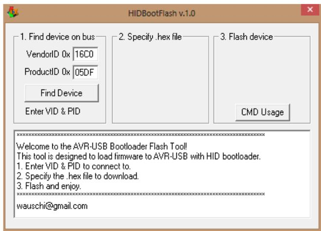
Fig. 9 HID Boot Flash for burning the code on the microcontroller
