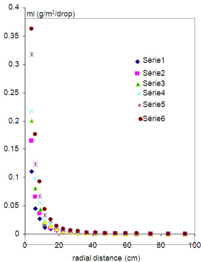
Fig. 6 The relationship between the splashed mass  $m_i$  ( $\text{g/m}^2/\text{drop}$ ) in the compartments and the radial distance for different slope angles. [serie1: 0°, serie2: 2°, serie3: 5°, serie4: 10°, serie5: 17° and serie6: 20°]
