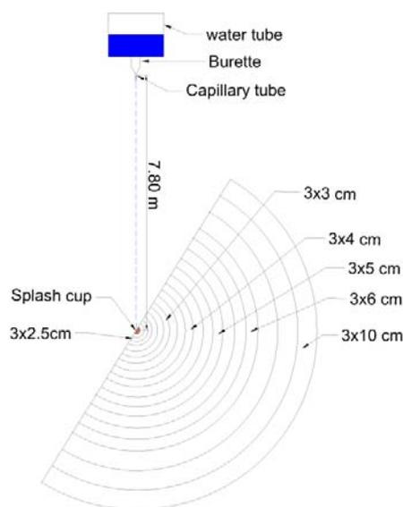
Fig. 4 General view of the splash board
