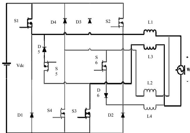
Fig. 2 Active stage of positive half line cycle
