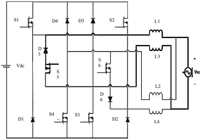
Fig. 3 Freewheeling stage of positive half line cycle
