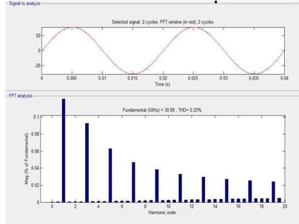
Fig. 12 Output current THD of proposed inverter
