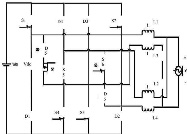
Fig. 1 Proposed transformerless inverter configuration
