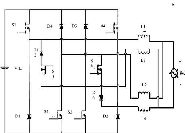
Fig. 5 Freewheeling stage of negative half line cycle
