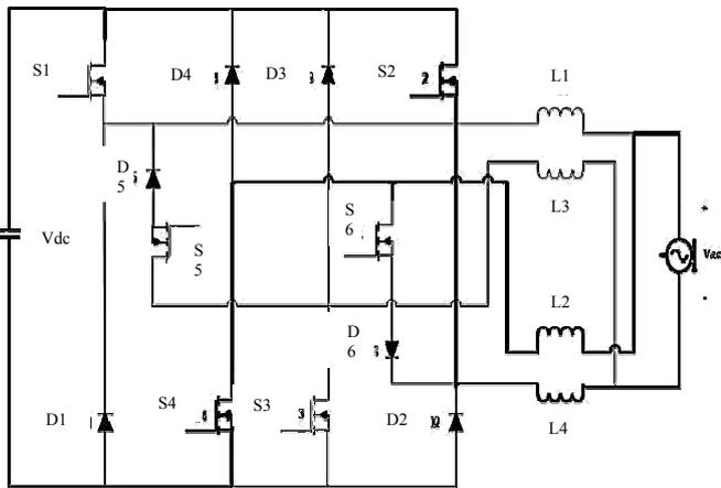
Fig. 4 Active stage of negative half line cycle
