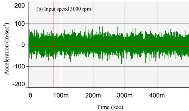
Fig.6 Time domain for the faulty gear (pitting of tooth) in fifth speed at 2000, 3000 rpm, input/output load 130/402 Nm
