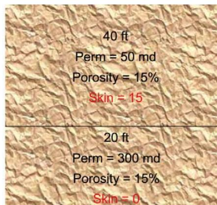
Fig. 1 (b) After acid treatment (without diverter)
