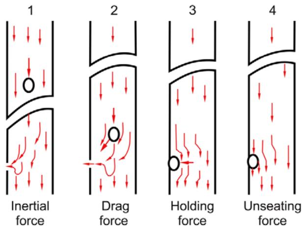
Fig. 2 Basic forces governing ball sealer efficiency [10]
