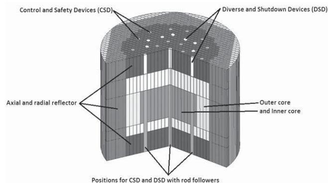
Fig. 1 3D cross-sectional view of GFR2400 reactor model
