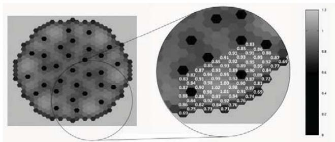
Fig.10 Spatial distribution of  $LMF$  in "All down" case with 1<sup>st</sup> and 2<sup>nd</sup> reflector ring withdrawn
