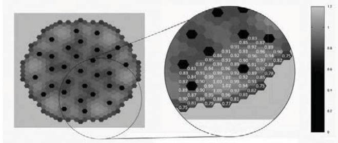
Fig.9 Spatial distribution of  $LMF$  in "All down" case with 1<sup>st</sup> reflector ring withdrawn
