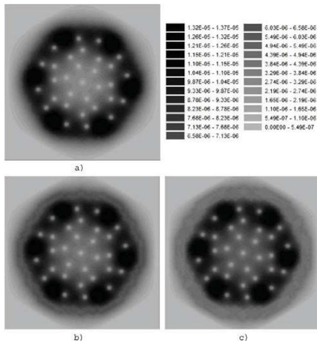
Fig.11 The spatial distribution of neutron fluxes for (a) "All down" case, (b) "All down" case with 1<sup>st</sup> reflector ring and (c) "All down" case with 1<sup>st</sup> and 2<sup>nd</sup> reflector ring
