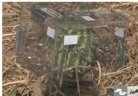
Fig. 8 A watermelon inside the Mechanical Force Gauge in farm
