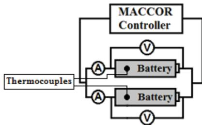
Fig. 1 Schematic of the battery connections for experiments
