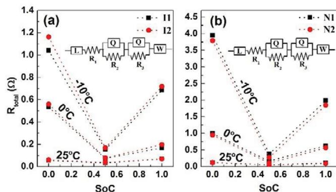
Fig. 4 Extracted resistance ( $R_{total}=R_1+R_2+R_3$ ) of battery from EIS test (a) INR type (b) NCR type battery. The inset shows the fitted curve of equivalent electrical circuit on experimental data (The dotted lines were drawn to determine the temperature)
