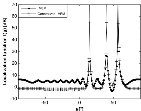
Fig. 5 One dimensional localization, SNR = 5dB
