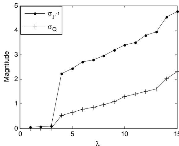
Fig. 4 Eigenvalues of MVDR and proposed operator
