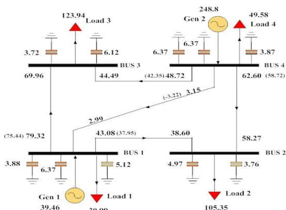
Fig. 2 Power flow diagram of 4 bus system
