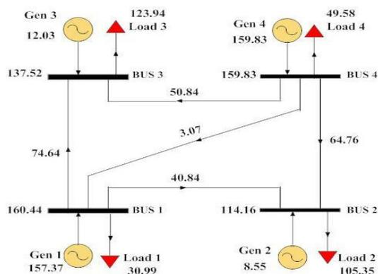
Fig. 3 Lossless Network of 4 bus system
