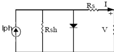
Fig. 2 Equivalent circuit of PV cell
