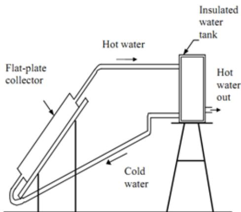
Fig. 1 Experimental setup of a single phase thermosyphon solar water heater with insulated water tank
