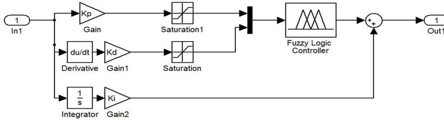
Fig. 1 Hybrid FLC controller block diagram
