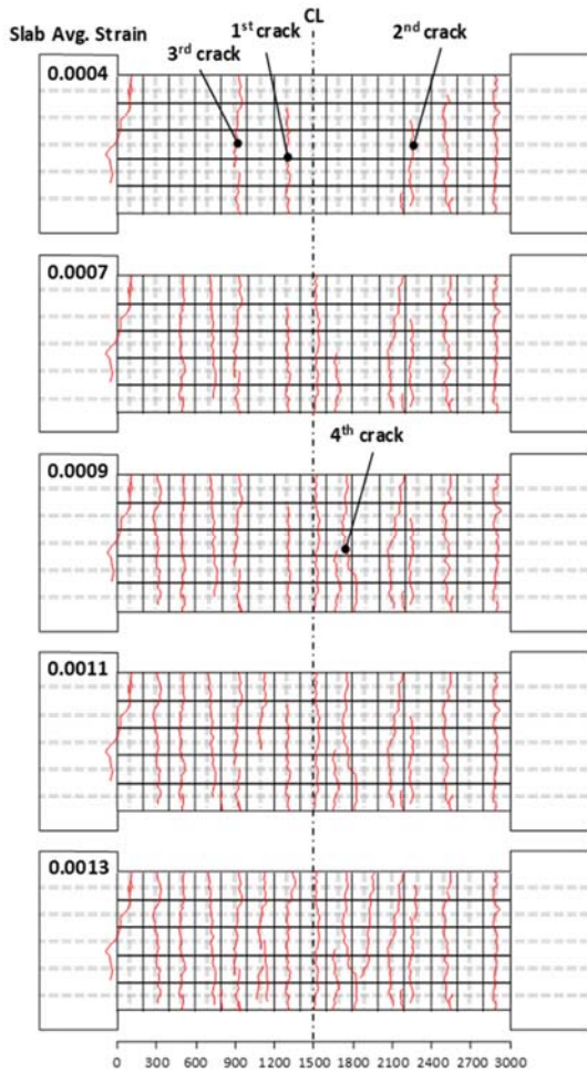
Fig. 7 The cracking pattern (specimen 3)
