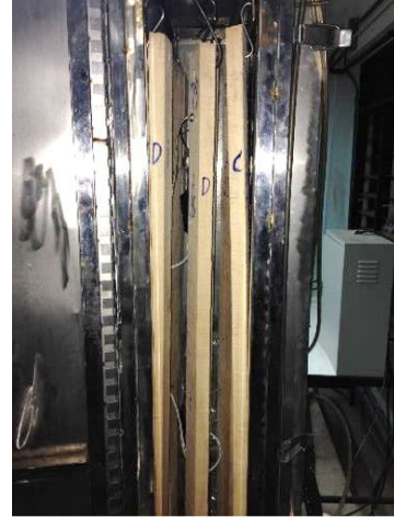
Fig.3 Wood samples and loadcell measurement weight loss.
