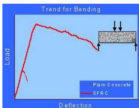
Fig. 2 Load vs Deflection for Plain Concrete & SFRC
