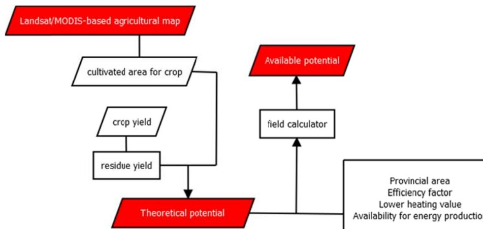
Fig. 3 GIS-based biomass resource assessment workflow
