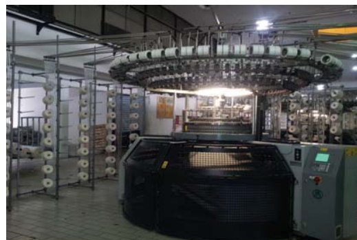
Fig. 1 Mayer and Cie weft knitting machine
