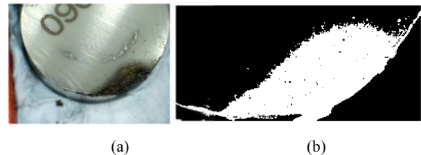
Fig. 8 Ceramic insert's crater wear area extraction with image processing (a) original image, and (b) processed worn area
