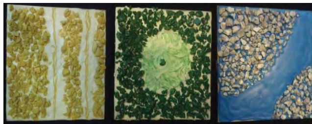
Fig. 1 Recycled concrete façade with different designs [18]
