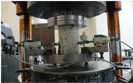
Fig. 3 Uniaxial compression test setup
