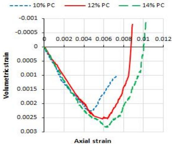
Fig. 7 Volumetric strain versus axial strain curve for PC specimens with different epoxy resin ratios including 10%, 12% and 14%
