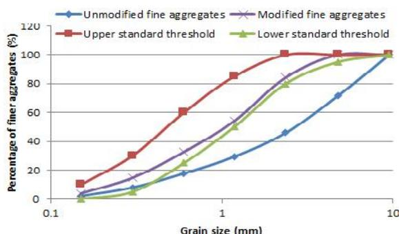
Fig. 1 Fine aggregate size distribution
