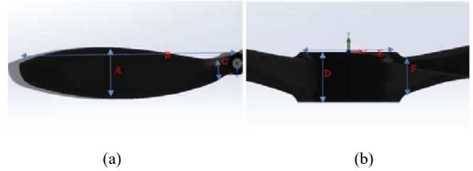
Fig. 3 Diagram of the Gemfan 1147 CAD model with annotated dimension locations shown in Table I, (a) View from top, (b) View from front
