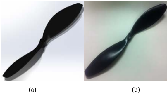
Fig. 2 Gemfan 1147 propeller shape identification: (a) CAD Model of Gemfan 1147, (b) Actual Gemfan 1147 propeller
