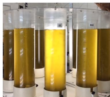
Fig. 2 Photo-bioreactor (patent: Privilege of Innovation, registration No. 0000221105500270)
