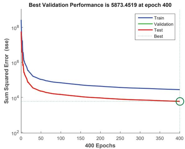
Fig. 7 Training performance in terms of SSE [deg<sup>2</sup>/samples] over 400 training epochs using [20] NN on simulated data and TS #2
