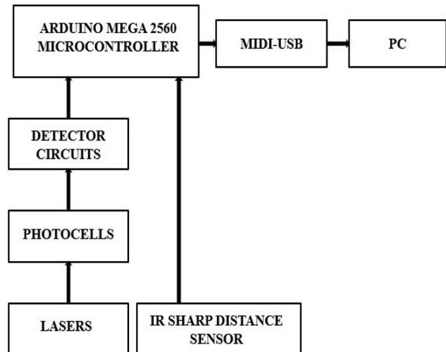
Fig. 2 Block Diagram of the proposed system
