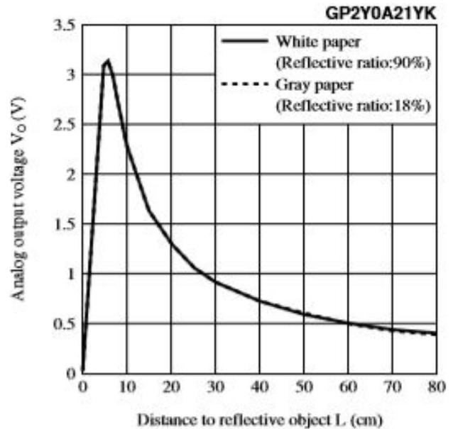
Fig. 8 Sensor Output (Voltage versus Distance to Object)
