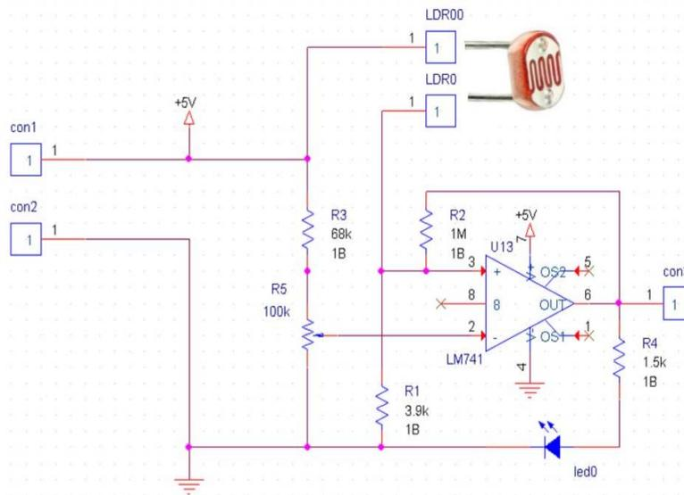
Fig. 5 Detailed internal circuit of detector module
