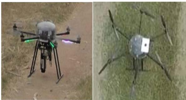
Fig. 3 UAV-LiDAR system used in this study
