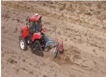
Fig. 8 Building bumps and hollows using a plough
