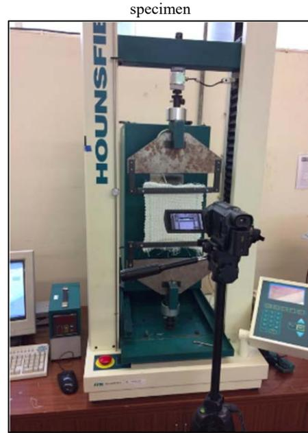
Fig. 6 Setup of testing Poisson's ratio
