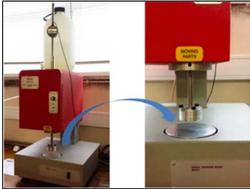
Fig. 4 Measurement of thickness of produced fabrics
