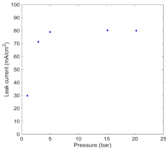
Fig. 8 Leak current vs pressure for a stack tested at 50% H<sub>2</sub>O + 50% H<sub>2</sub> on fuel electrode and air on oxygen electrode
