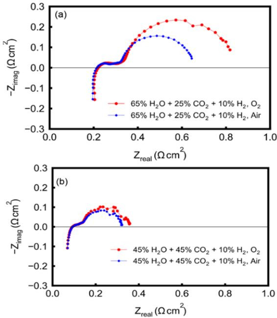
Fig. 2 Gas shift analysis on oxygen electrode under co-electrolysis conditions (a) Cell type-E with 65% H<sub>2</sub>O + 25% CO<sub>2</sub> + 10% H<sub>2</sub> on the fuel electrode, (b) Cell type-B with 45% H<sub>2</sub>O + 45% CO<sub>2</sub> + 10% H<sub>2</sub> on the fuel electrode
