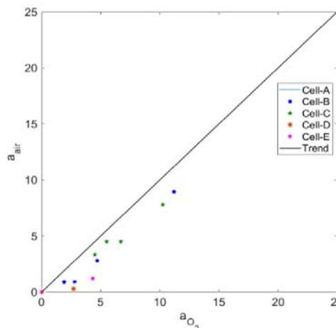
Fig. 7 Values of  $a$  in air are plotted vs  $a$  in oxygen for all the cells analyzed under steam and co-electrolysis conditions (Cell-A line overlaps with the trend completely)
