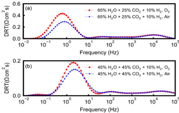
Fig. 3 DRT analysis with a shift from oxygen to air on the oxygen electrode under co-electrolysis conditions (a) Cell type-E with 65% H<sub>2</sub>O + 25% CO<sub>2</sub> + 10% H<sub>2</sub> on the fuel electrode, (b) Cell type-B with 45% H<sub>2</sub>O + 45% CO<sub>2</sub> + 10% H<sub>2</sub> on the fuel electrode
