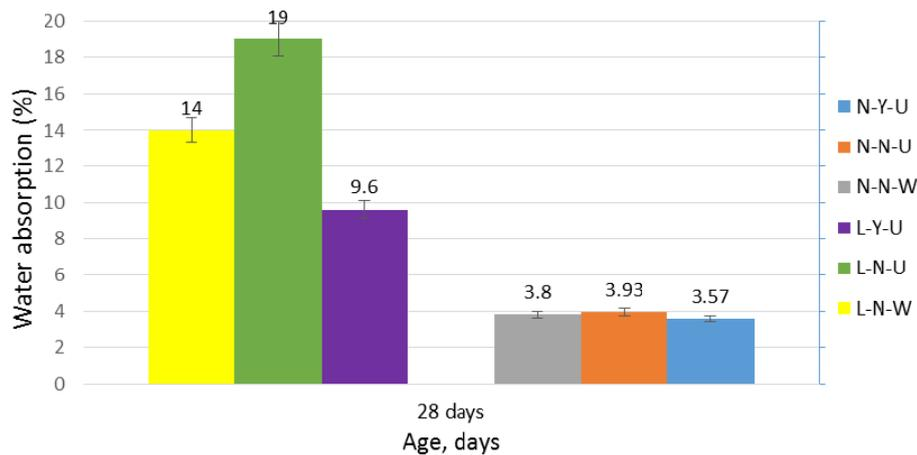
Fig. 2 Water absorption of concrete specimens at 28 days
