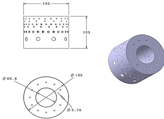
Fig. 3 Geometrical model of the combustor liner
