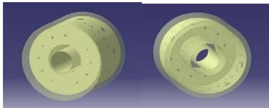
Fig. 5 Fluid domain of the combustor
