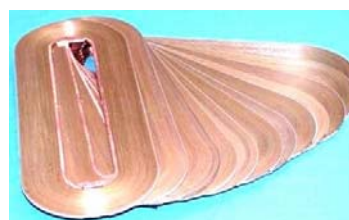
Fig. 6 An example of pancake coils
