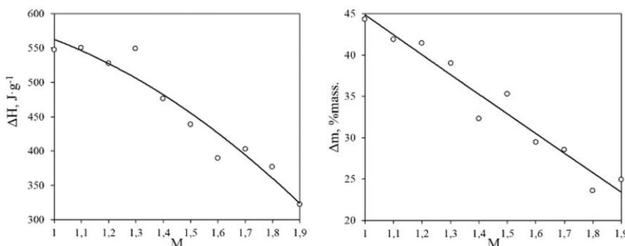
Fig. 9 Dependences of the quantity of released heat and mass loss in the process of ammonium nitrate exothermal decomposition on the molar ratio (M)
