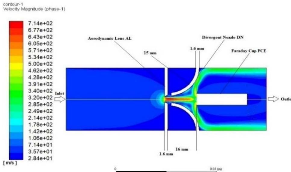
Fig. 6 The main parts used for our study
