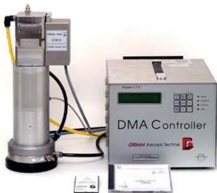
Fig. 3 Differential mobility analyzer
