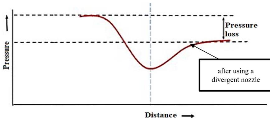
Fig. 12 The diagram shows the relationship between pressure and the distance after using a divergent nozzle
