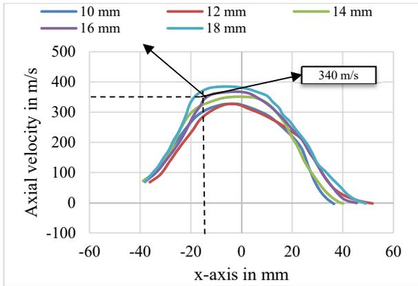
Fig. 5 The axial velocity along the x-axis with the length of the section between the lens ( $x = 0$ ) and FCE being  $x = (10 \text{ mm}, 12 \text{ mm}, 14 \text{ mm}, 16 \text{ mm}$  and  $18 \text{ mm})$
