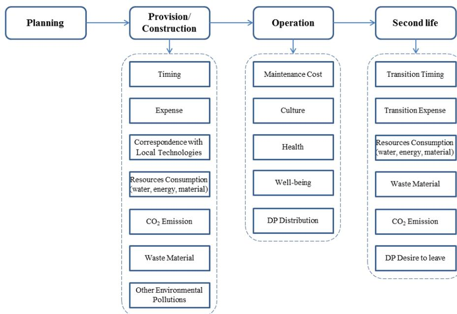
Fig. 3: Life cycle phases of TH from cradle to grave and associated indicators
