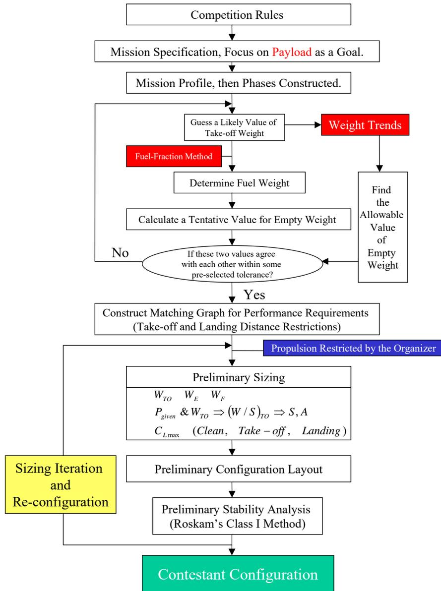
Fig. 1 Mini UAV design process
