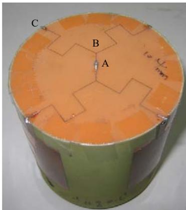
Fig. 6 Feed network of 1 × 4 array
