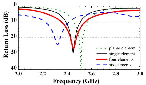
Fig. 8 Measured return loss for low-profile antenna of 1 × N array
