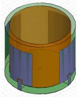
Fig. 5 Design of low-profile omni-directional antenna on UAV
