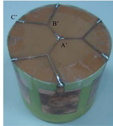
Fig. 7 Feed network of 1 × 6 array
