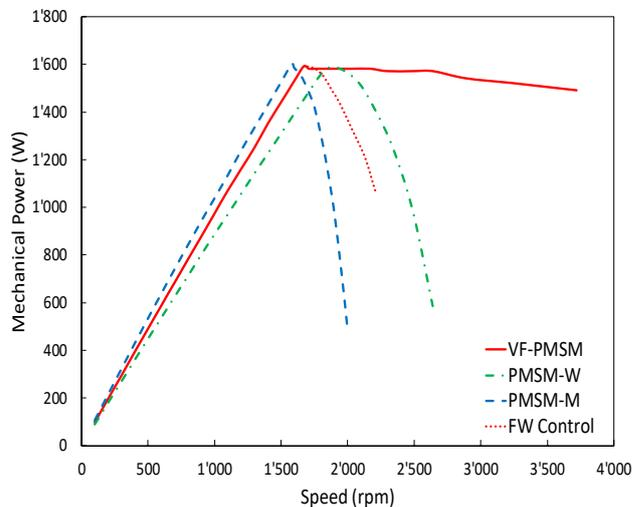
Fig. 14 Measured mechanical power of PMSM
