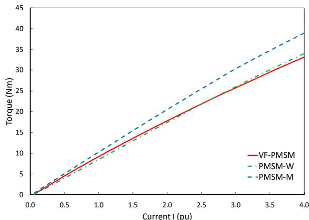
Fig. 15 Comparison of measured characteristics torque-current at 100 rpm
