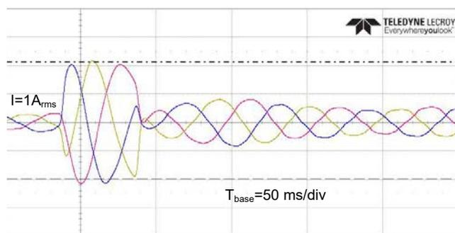
Fig. 10 Transient stator currents in demagnetization process
