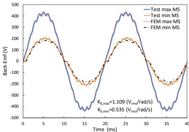
Fig. 7 Measured phase-to-phase no-load voltage at 1500 rpm
