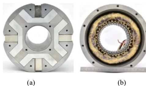
Fig. 5 (a) Rotor of VF-PMSM; (b) 36-slots stator
