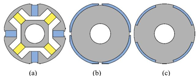
Fig. 1 Rotor's topologies: (a) VF-PMSM; (b) PMSM-M; (c) PMSM-W
