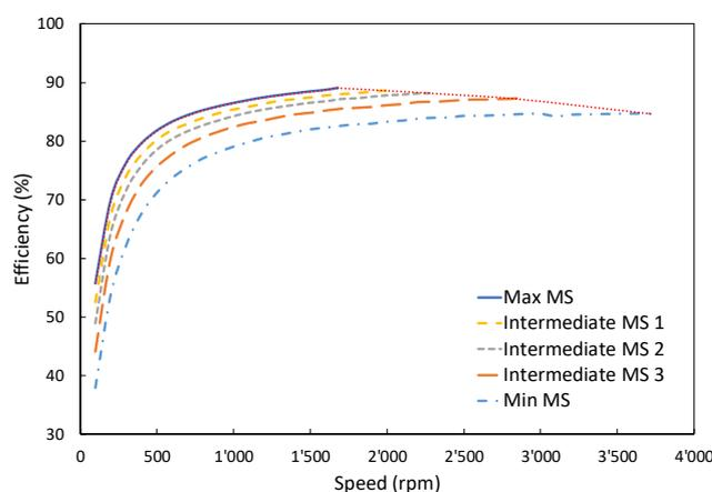
Fig. 12 Measured motor efficiency for different magnetization states
