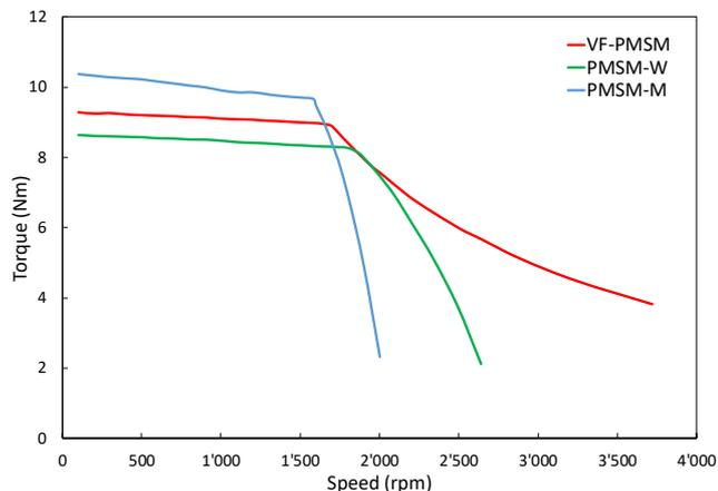
Fig. 13 Measured torque-speed characteristics of PMSM under nominal current (VDC = 600 V)
