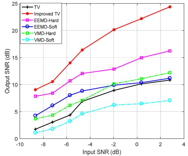
Fig. 5 The variation of the output signal-to-noise ratio (SNR) by EEMD, VMD, TV and the improved TV methods. The improved TV method outperforms other methods.
