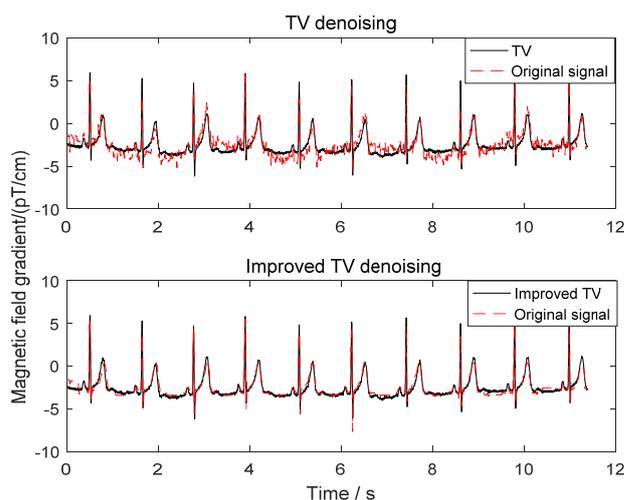
Fig. 3 A comparison of the original signal (dotted line) with the reconstructed signals (solid line) obtained from TV based denoising method and the proposed method is shown in the figure
