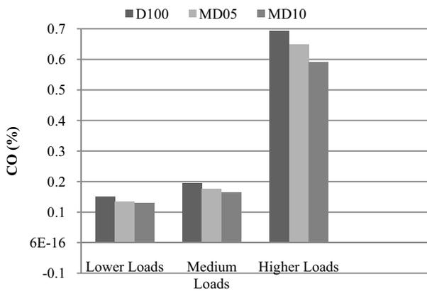
Fig. 9 Emission of CO at various loads
