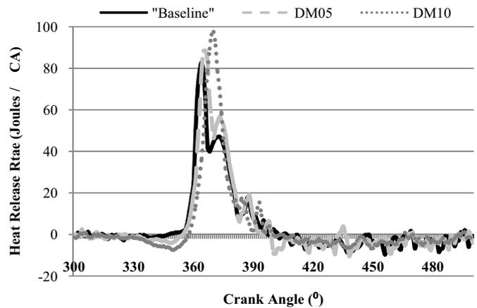
Fig. 4 Heat release rate diagram for test fuels
