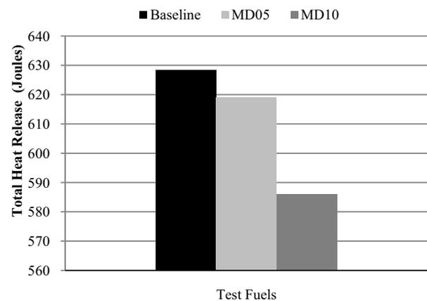
Fig. 8 Total cyclic heat release in Joules
