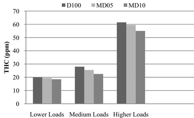
Fig. 10 Emission of THC at various loads
