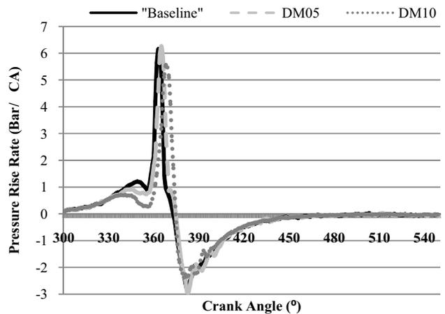
Fig. 3 Pressure rise rate diagram for test fuels
