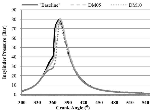
Fig. 2 Pressure-crank angle diagram for test fuels
