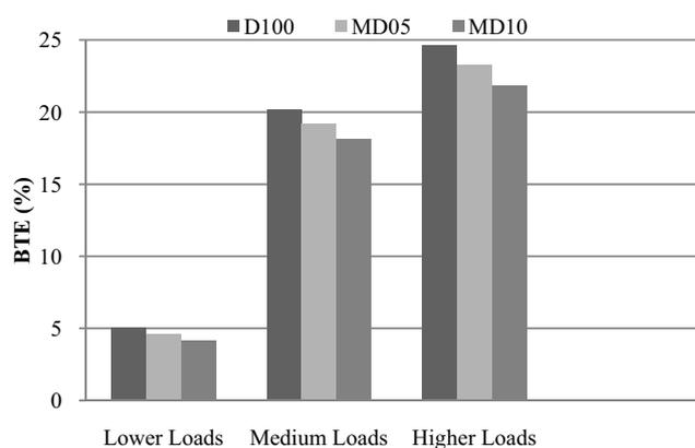
Fig. 14 BTE for test fuels at various loads
