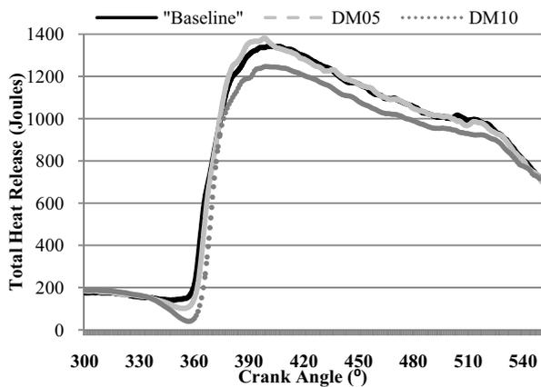
Fig. 5 Cumulative heat release for test fuels
