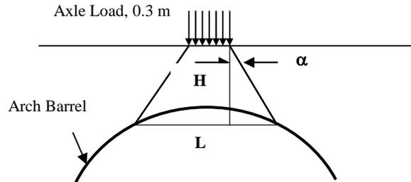
Fig. 12 Axle Load Distribution through the Fill Material
