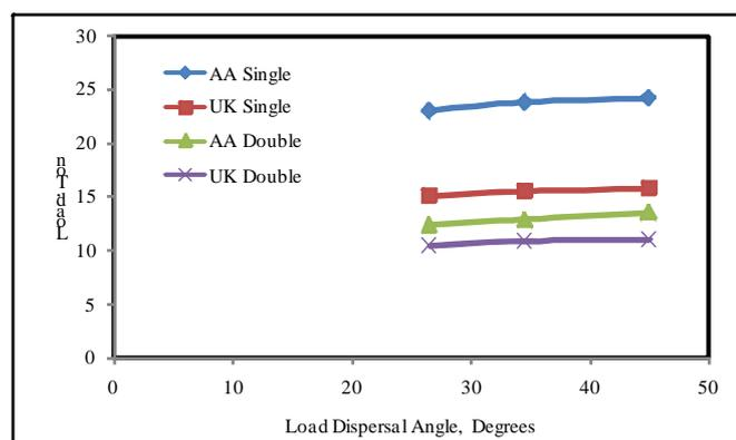
Fig. 3 Load vs Dispersal Angle, Killeen Bridge
