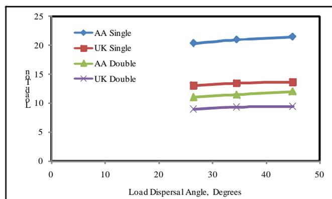
Fig. 2 Load vs Dispersal Angle, Griffith Bridge
