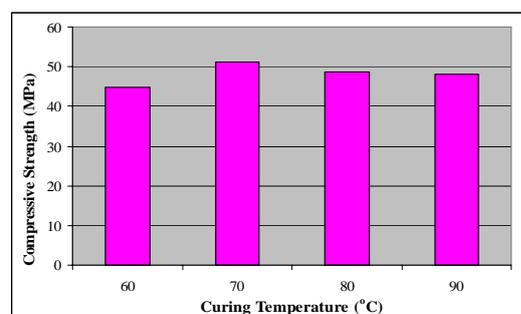
Fig. 7 Effect of Curing Temperature on Compressive Strength
