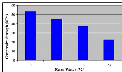
Fig. 5 Effect of Extra water on Compressive Strength
