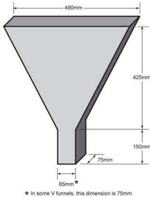
Fig. 2 V-Funnel Apparatus
