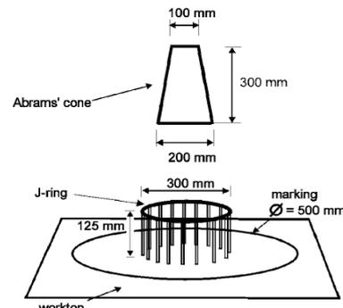
Fig. 4 J-Ring Test Apparatus
