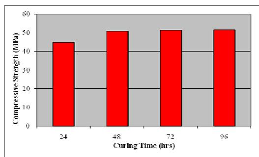
Fig. 6 Effect of Curing Time on Compressive Strength
