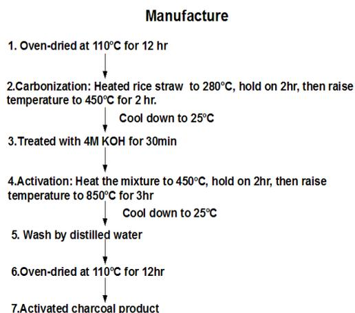
Fig. 1. Procedure for the preparation of activated carbon
