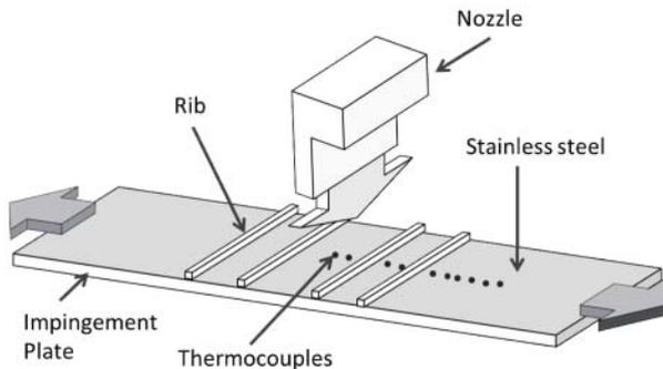
Fig. 2 Schematic diagram of the rib wall
