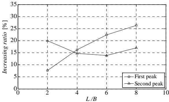
Fig. 11 Increasing heat transfer ratio at  $H/B=15$ ,  $L_1/B=4$
